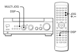
The DSP (Digital Signal Processor) surround circuits can recreate the effect of sounds reflected from walls or ceilings, to obtain the sound presence of real environments. The unit provides 5 DSP preset modes.
